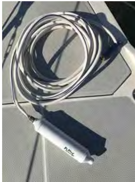
Hose and filter used to fill water tanks at the dock.
