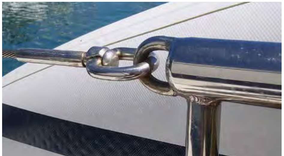
Here I cut off the top rail, leaving about 1/2" past the stanchion to cap off with a small piece of flat stainless sheet and welded a loop on for the lifeline closure cables.
