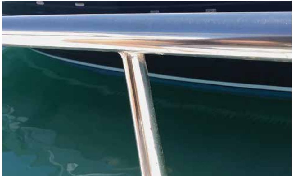
I TIG welded from the front and worked my way aft until I reached the last stanchion at the companionway.
