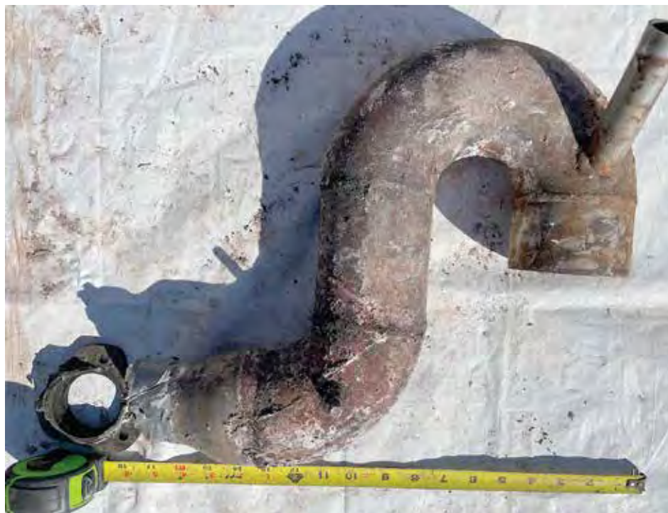
Exhaust Elbow after Removal – As viewed from front/bow end when mounted on engine
