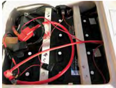
The SG200 shunt is in the back between the two hold down bars. Note battery terminal caps.
