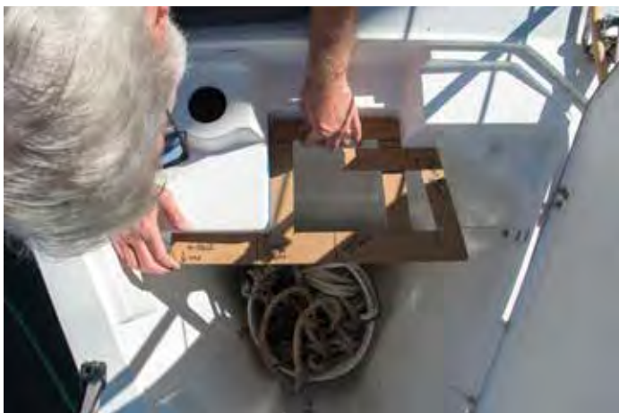
Making the template for the windlass support shelf. I used 1/8" MDF and a hot melt glue gun to determine the shape of the shelf.
