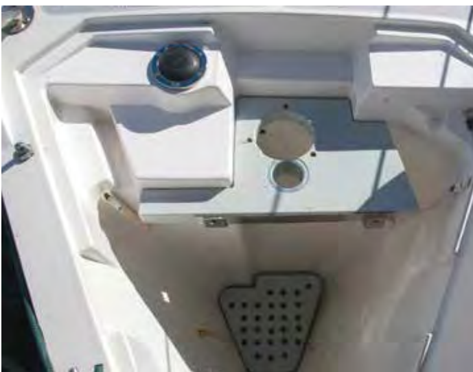
The shelf in place. Note the galvanized collar in the chain drop hole, the PVC holder for the windlass break Allen wrench to the left of the shelf and the raised floor in the bottom to the chain locker to keep the rode out of any water in the locker.
