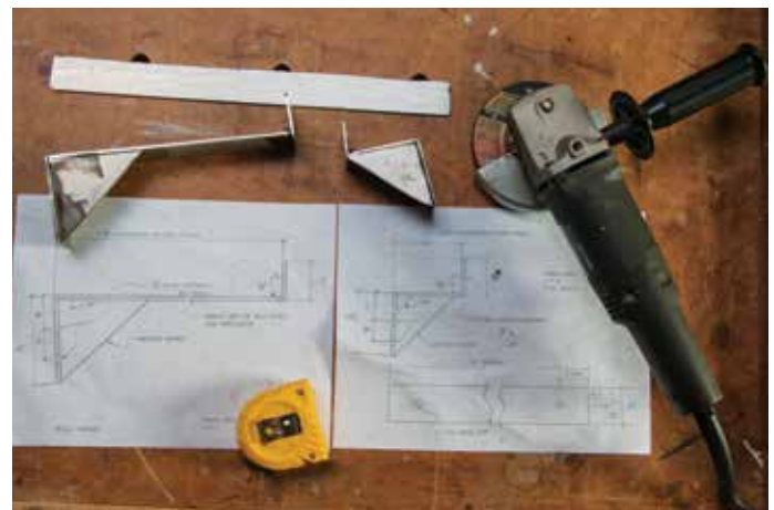
Rough plans for the brackets and the actual brackets after the first bit of clean-up.
