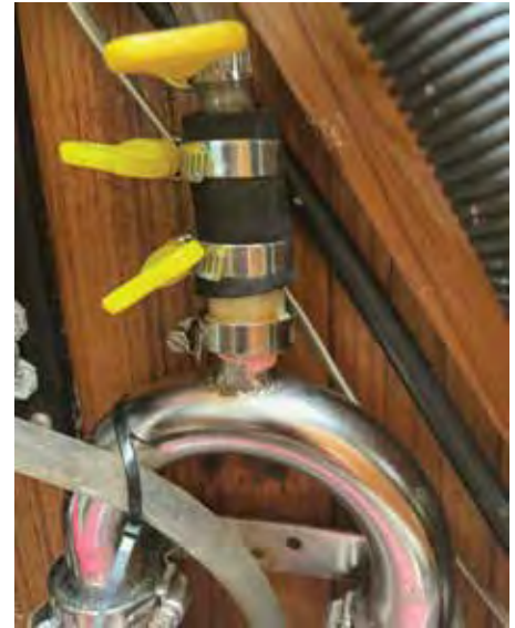
Engine vented loop drip catcher for leaking vacuum break valve. Carries slow drips through a hose from faulty valve to bilge to prevent water damage to engine compartment. Photo by Joe Rocchio.
