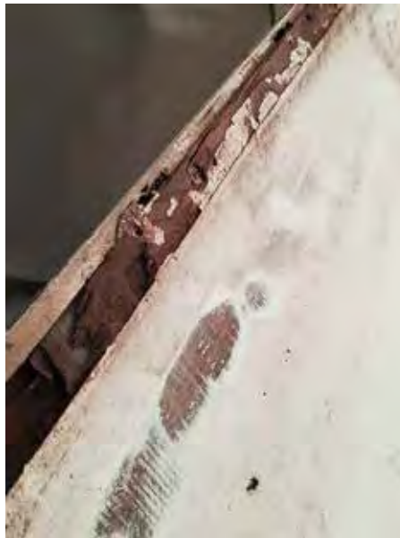
Rotted wood core at edges of sea hood. You can also see the wear mark from the hatch rubbing.
