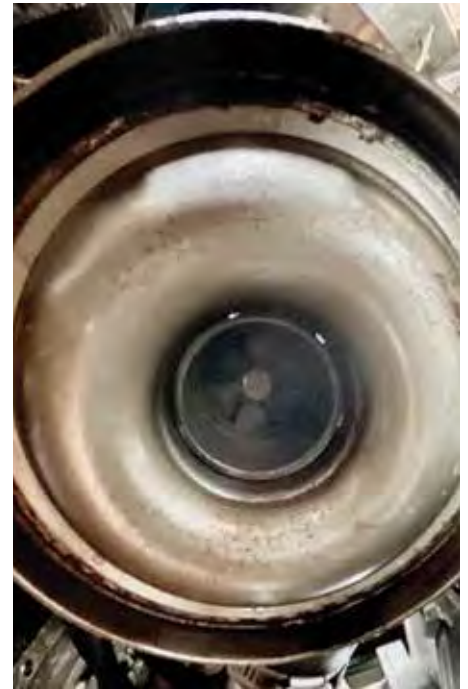
Air intake to turbocharge on a 4JH3TE engine with the filter can cover removed.
