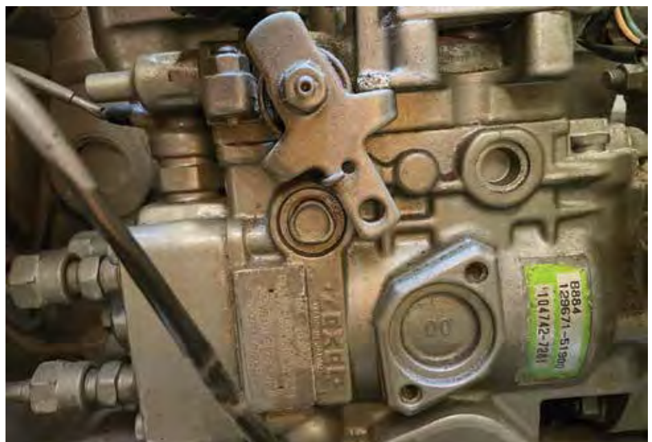
Stop lever on fuel control system. Rotate clockwise momentarily to stop engine.
