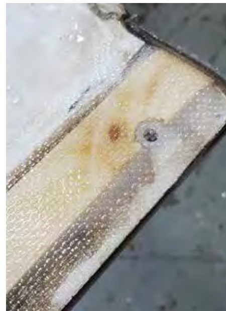
Wood with first layer of 2 inch woven tape
