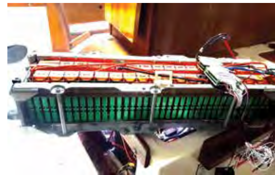
Battery pack for a total of 48V and 14 kW-h of capacity.
