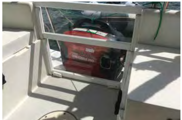
The second insert in-place with the generator on the walk-off step. Aside from blocking exhaust from coming back into the cockpit it also makes it a little quieter down below when the generator is running.
