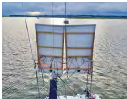
600 Watts of solar panels on the custom frame. The panels rotate to follow the altitude of the sun and maximize charging.
