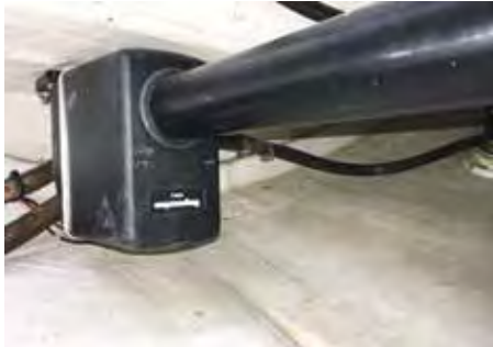
e) Raymarine Actuator Control Unit: Product #E70099 was installed under the heads sink unit. Taking-out the locker doorframe provides better working access to install the ACU.
