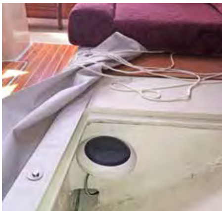
f) Raymarine Sensor Core: Product #E70096 was positioned in the starboard locker forward of the Holding Tank as we wanted to keep it clear of any electro-magnetic interference. Looking back, I think we were a bit over-cautious and this could have been installed below the head sink along with the ACU. [ Tech Ed note – With any sensor that contains magnetic sensing functions, constant vigilance is required to be aware of what is stored or located anywhere in close proximity to such a sensor that might be magnetic. A bit
