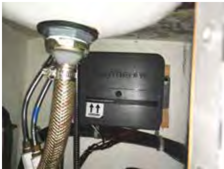
f) Raymarine Sensor Core: Product #E70096 was positioned in the starboard locker forward of the Holding Tank as we wanted to keep it clear of any electro-magnetic interference. Looking back, I think we were a bit over-cautious and this could have been installed below the head sink along with the ACU. [ Tech Ed note – With any sensor that contains magnetic sensing functions, constant vigilance is required to be aware of what is stored or located anywhere in close proximity to such a sensor that might be magnetic. A bit
